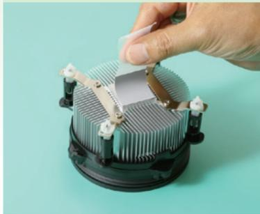
Apply onto Heat Sink
