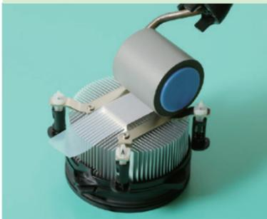
Roll twice on the film to attach to heat sink
